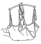
When the standard lifting hanger is placed perpendicular to the patient. The 3 (6) straps closest to the head of the patient are mounted in the hangers two lifting hooks closest to the head of the patient. Always mount the head straps at last. The 2 bottom straps are placed at the two hooks furthest from the head of the patient.
